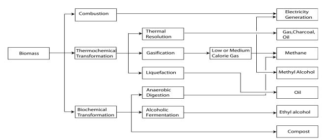
Fig.1 Energy Transformation Technology of Biomass
